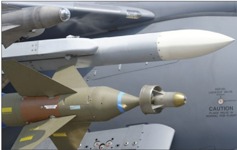
Typical non-penetrating munitions include aerial laser-guided bombs (top) and the laser-guided Mk 84 GP bomb (bottom). Although effective against surface targets, neither will penetrate reinforced bunkers. (Photo courtesy of author)
